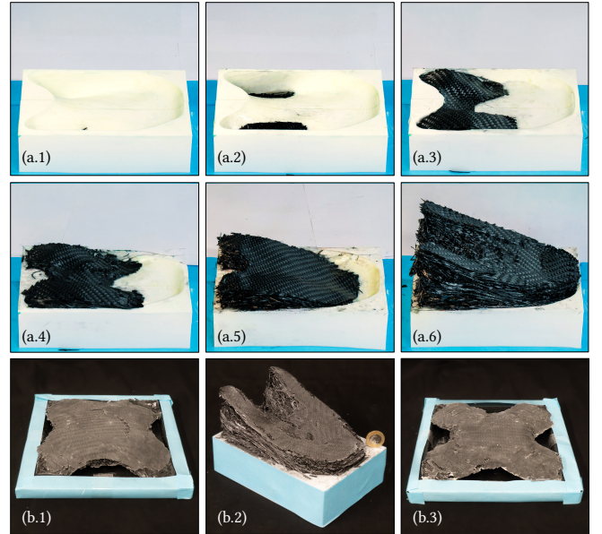
Fig. 13. The fabrication of laminated composites are taken on 3D printed moulds – see an example of fabrication sequence as illustrated in (a.1-a.6), and all the physically fabricated models are shown in (b.1-b.3).
